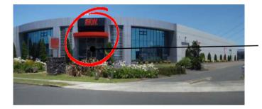
The main entrance is distinct and unmistakeable with a canopy, as well as colour/material change to the rest of the building. Basic signage is logically provided here.
