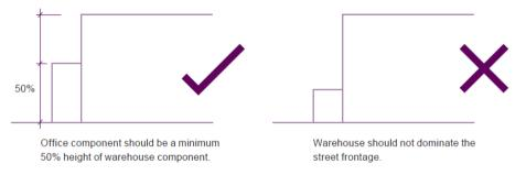
The total height of factory/warehouse component shall be no more than double the height of the office/administration component unless suitable architectural elements are included in the factory component.
